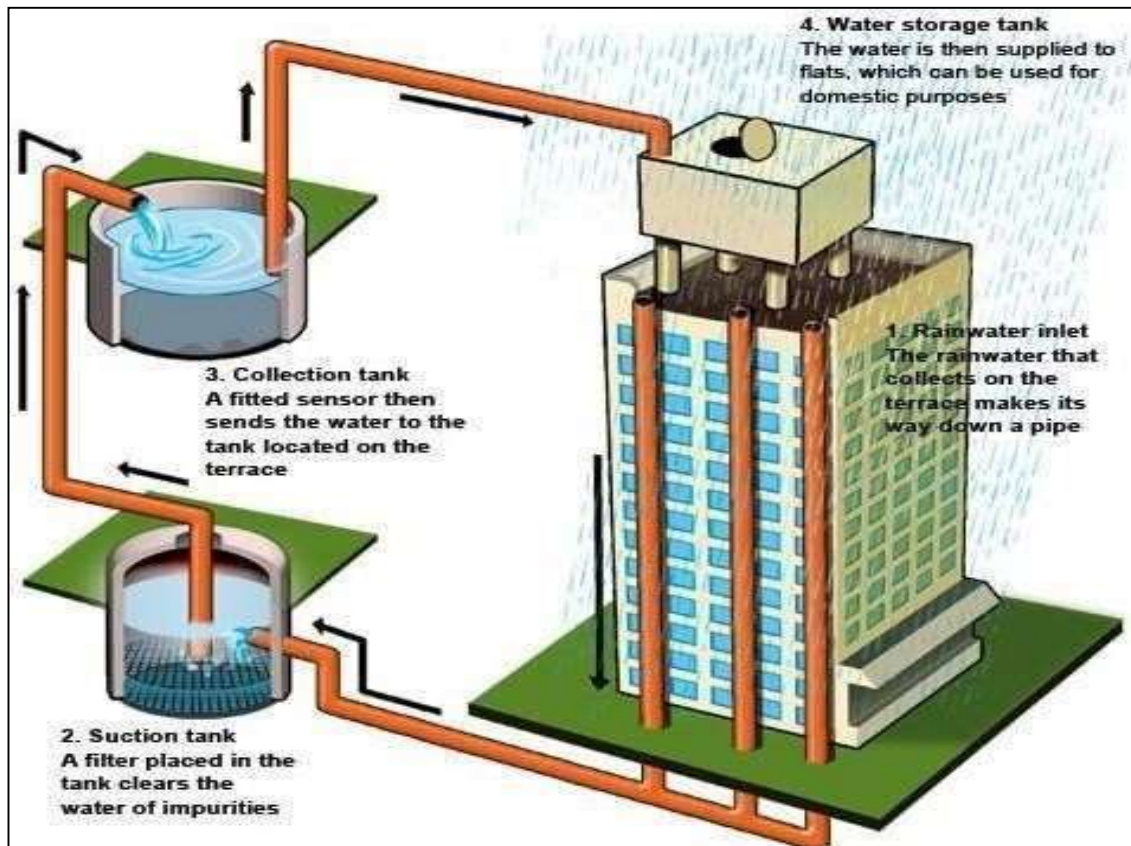
FIG.58: RAINWATER HARVESTING SYSTEM
